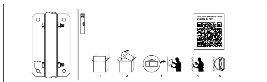
Each VOLCANO package has a printed template representing the spacing of boreholes and a leveling line to facilitate the mount of the console to the wall. Simply cut the template out of the cardboard lid and proceed to assembly.
