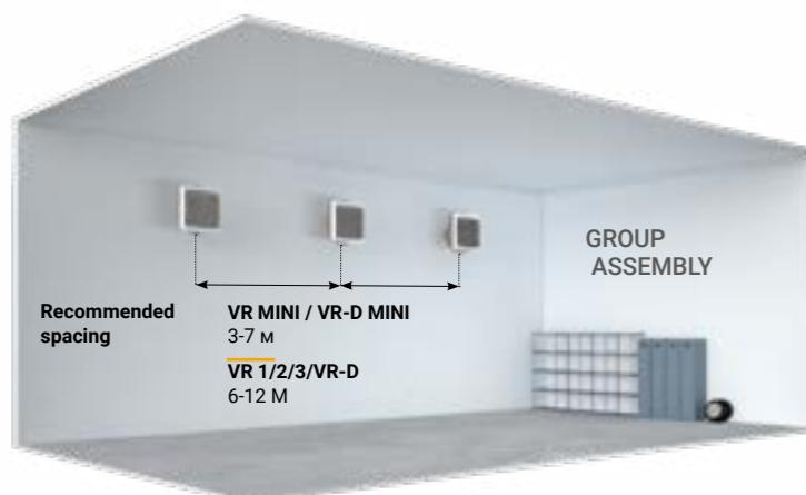
VOLCANO sets are equipped with a standard assembly console for wall and ceiling mounting of the device. The maximum vertical range of the devices is 8-15 m, depending on the type of heater. The maximum horizontal range of the devices is 14-25 m.
